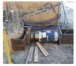
Lateral load test setup
