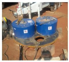
O-Cell Load plate assembly
